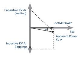
As the angle  $\emptyset$  is reduced,  $\cos \emptyset$  tends to 1 (unity power factor). Both apparent power (kVA) and total reactive power (kVAr) are significantly reduced.
